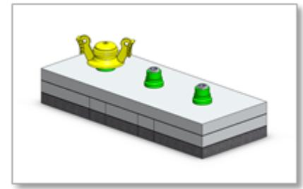
3. Slide the Kap (1) down around the bolt until sealant fills the Kap, comes out of the vent hole (3) and 360° squeeze out is achieved.
